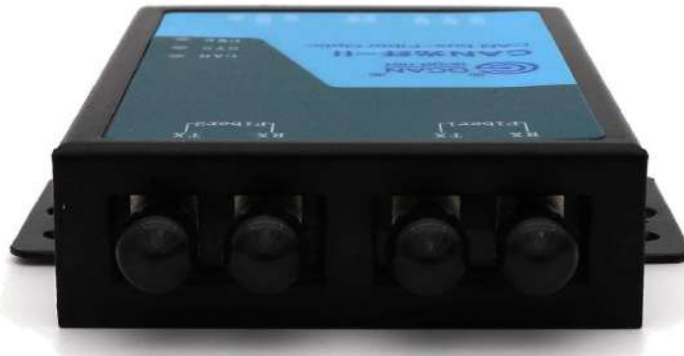
Figure 2.6 GCAN-208-2 fiber interface position
