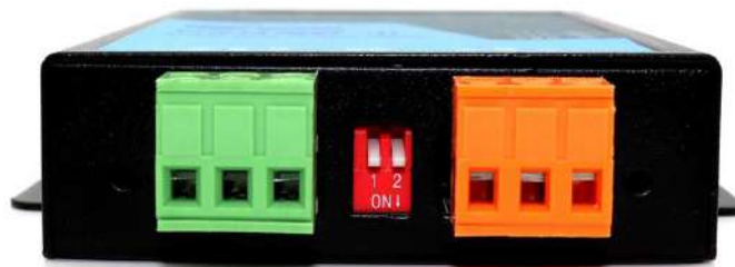
Figure 2.5 GCAN-208-2 CAN bus interface and power interface location
