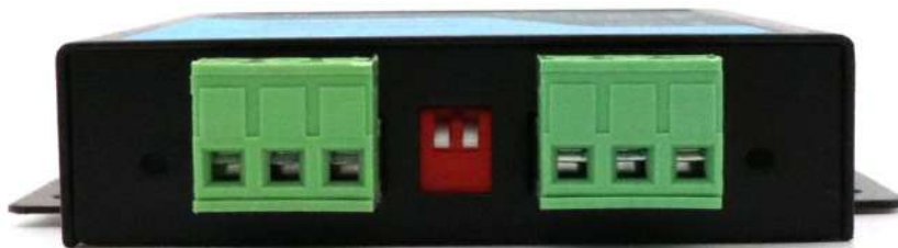
Figure 2.4 CAN bus interface of GCAN-208-1 module
